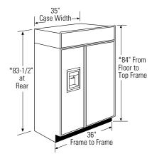
\*Shipping height. The refrigerator can be adjusted to fit into a cutout that is 83-1/2" min. to 84-1/2" max. height. Note that the top case trim at the front is 1/2" higher and will overlap upper cabinetry or soffit. Use leveling legs and wheels for height adjustment.
